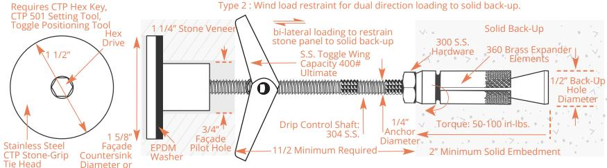
• S.S : ASTM 580A, Type 304; ASTM A-276
