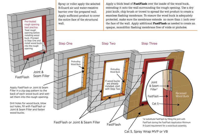
**Wood buck --** If wood bucks are not already installed, apply two thick beads of **FastFlash** or **Joint & Seam Filler** along the perimeter faces of the wood buck before attaching it to the structure while still wet. Install anchor bolts.
