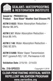
**NOTE**: The SWR Institute Validation Program uses standardized testing for validation purposes, including testing on CMU. PROSOCO <u>does not</u> recommend the use of Siloxane PD on CMU. Please reference the Substrate Chart on page 2.
