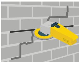
**STEP 1.** Grind away existing mortar, 20" minimum on each side of crack, 1-1/2"-2" deep. Clean with Water.
