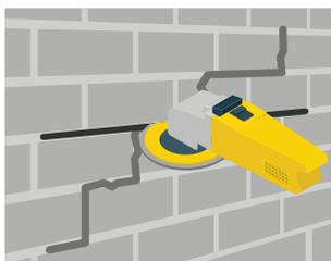
**STEP 4.** Apply second/third bead of SureGrout over Stitch-Tie Bar, and compact with appropriate trowel.
