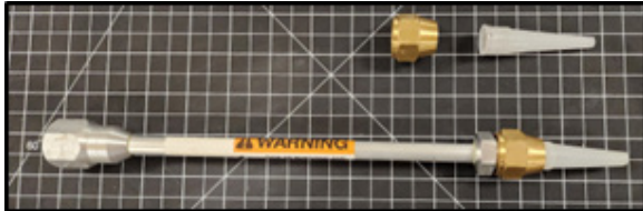
FIGURE 1: Spray gun equipped with extension wand, 5/8" flare brass rod nut, and caulk nozzle.
