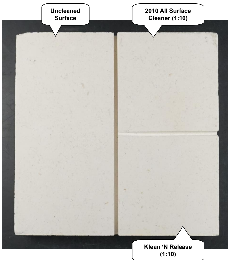
"Shellstone" Limestone After Cleaning
