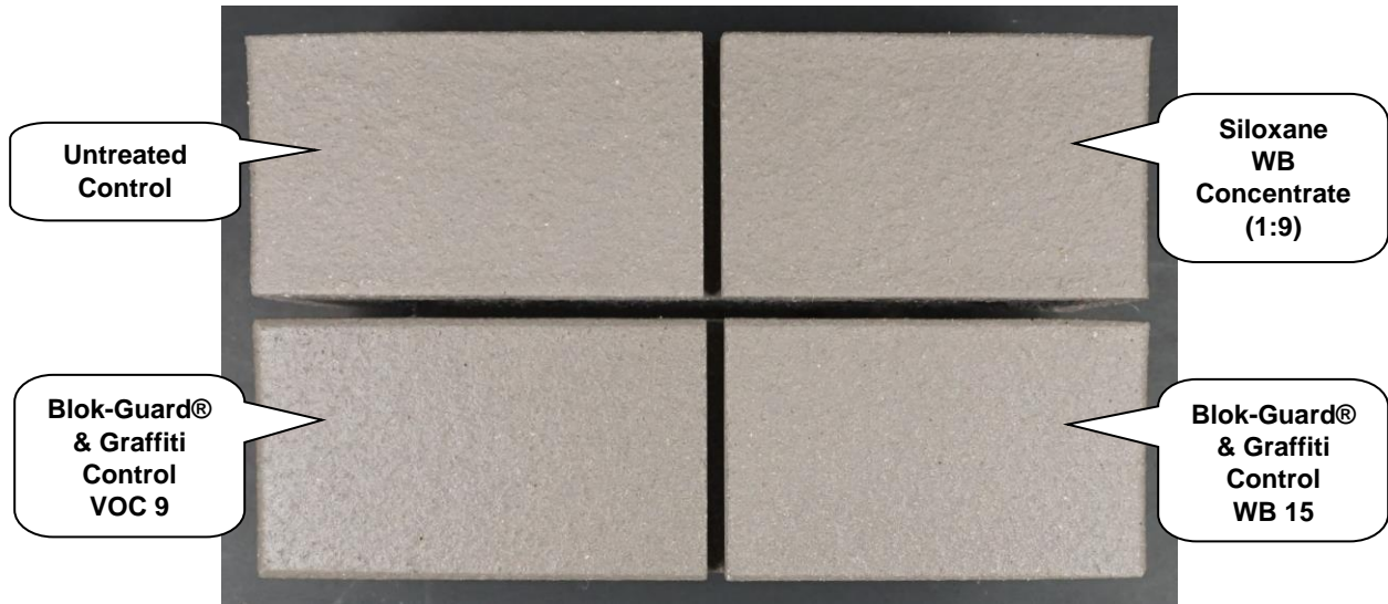
"Manhattan" Brick After Application
