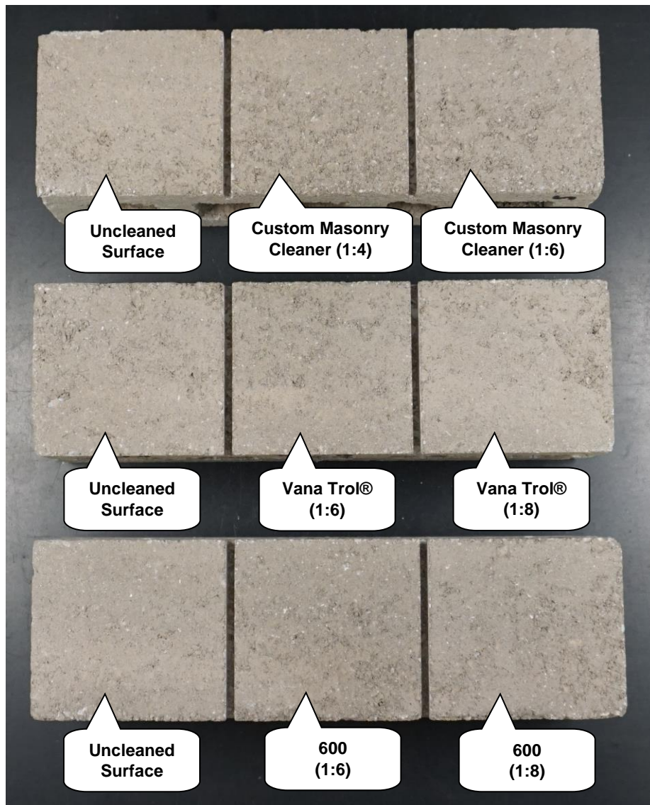
"Oakwood" Concrete Brick After Cleaning
