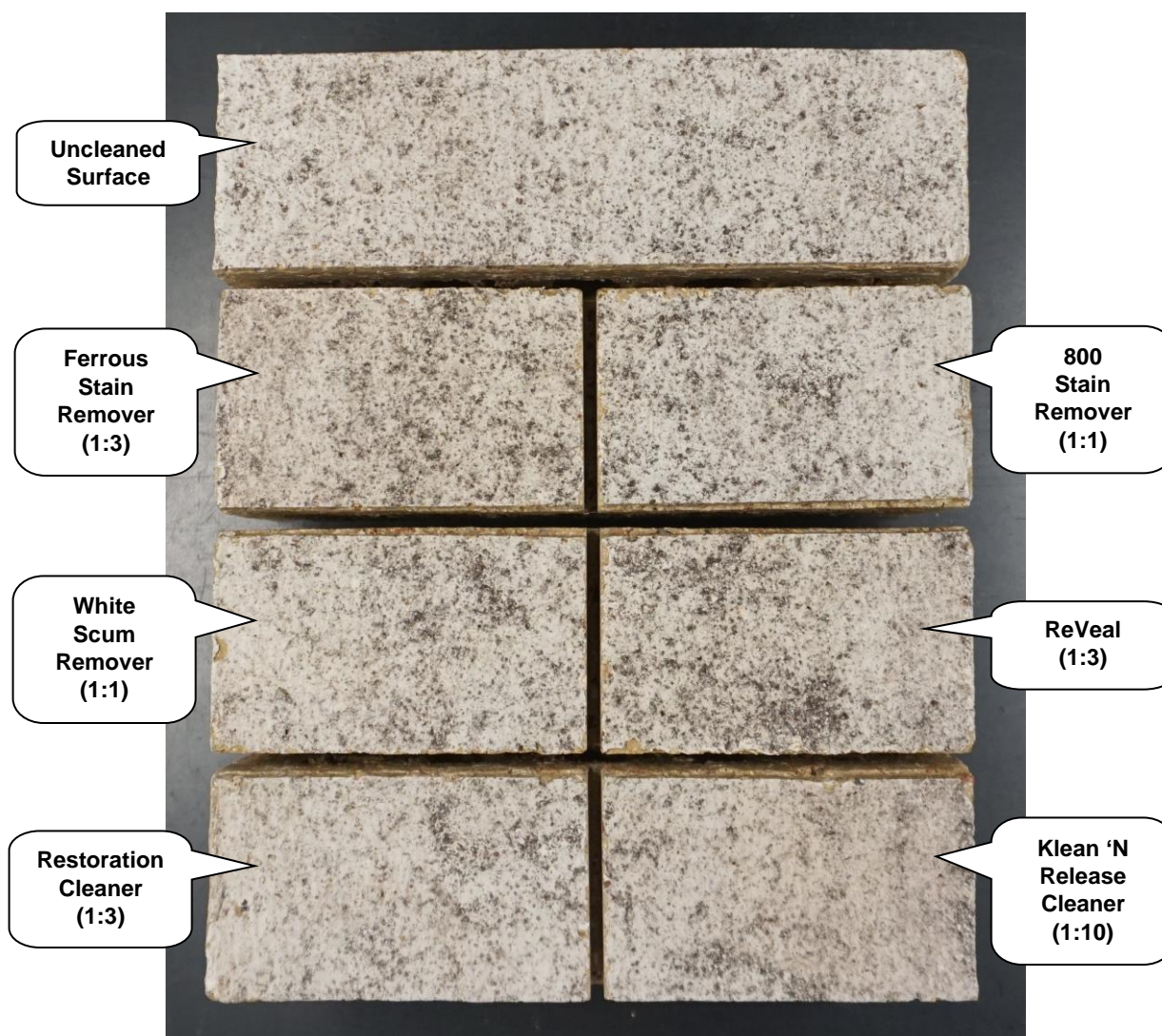
"Silverbrook" Modular Brick After Cleaning
