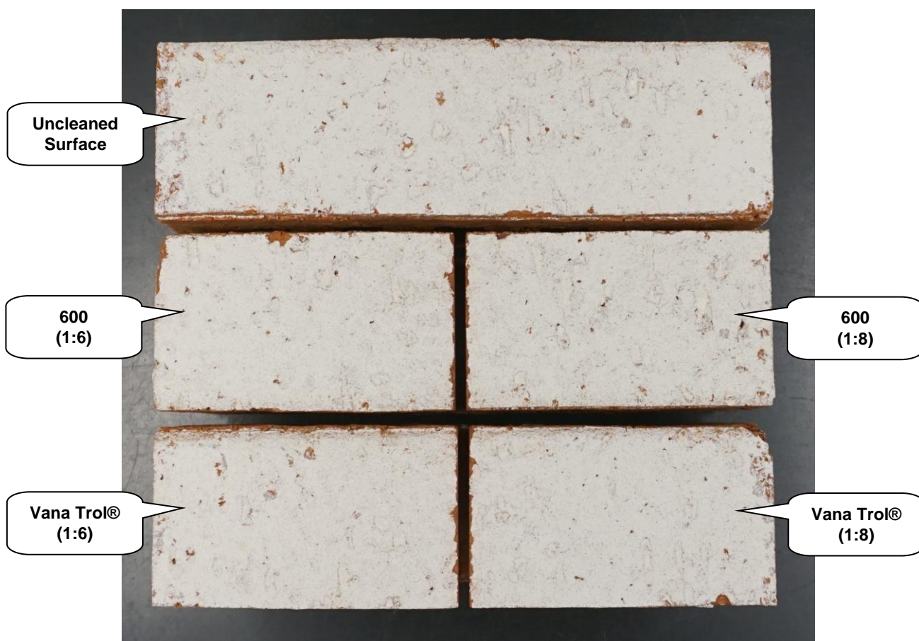
"Charter White" Modular Brick After Cleaning
