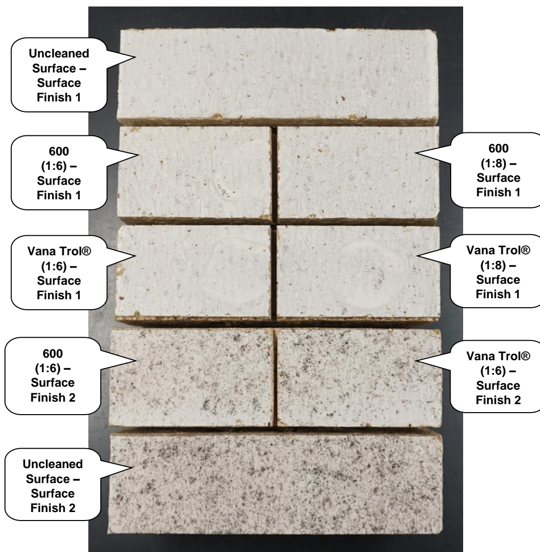
"Silverbrook" Modular Brick After Cleaning
