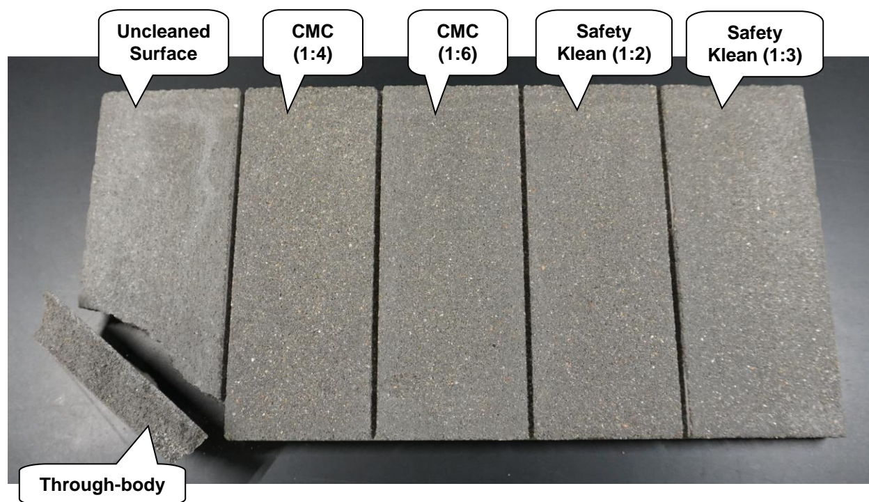
"Fine Smoke" Smooth Face CMU After Cleaning
