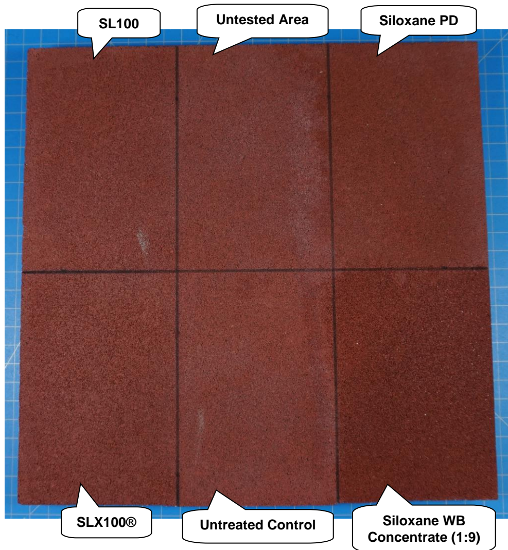
"# 25" Cast Stone With Treatments
