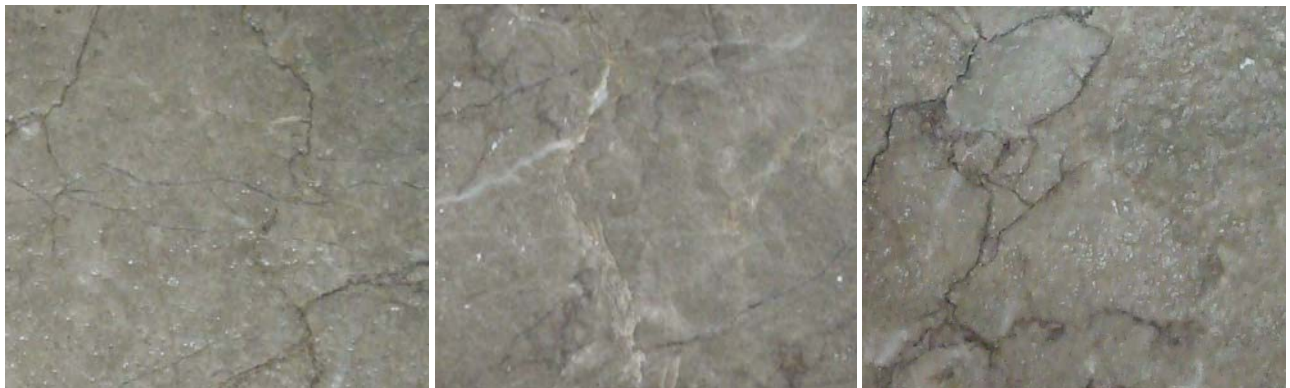
Stand Off® Stone, Tile & Masonry Protector (STMP) Untreated Control Stand Off® Limestone & Marble Protector
