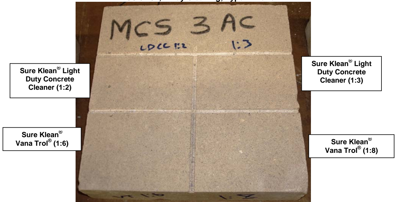
“MWCS 3AC”; 7 Day Cleaning; Type N Mortar
