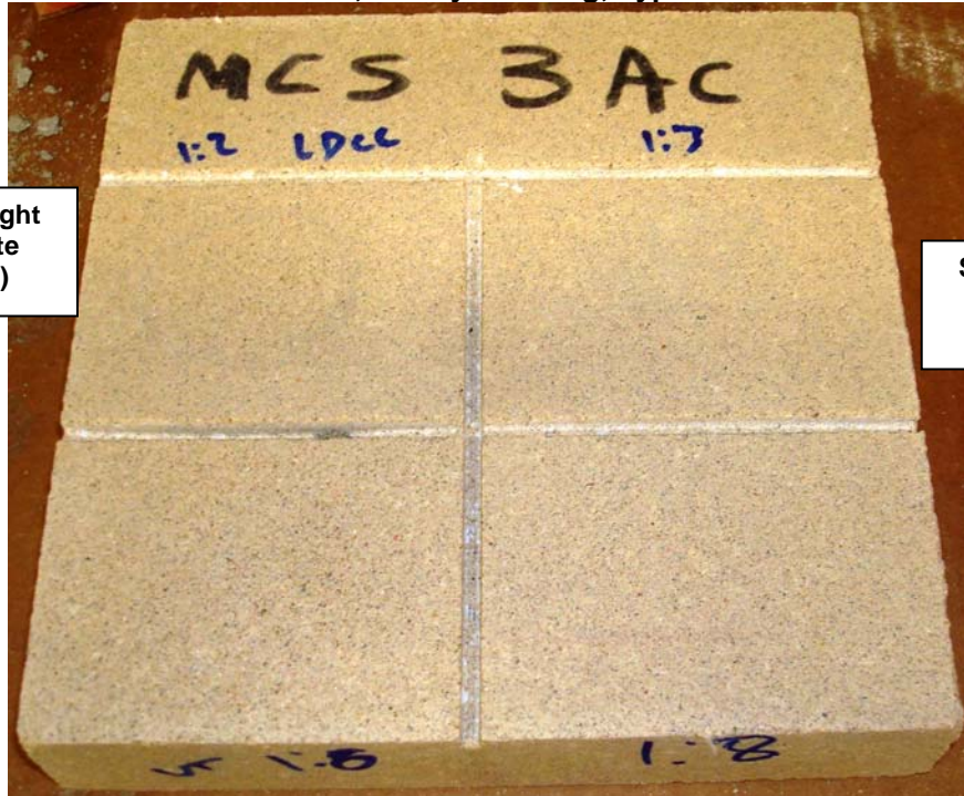
“MWCS 3AC”; 21 Day Cleaning; Type N Mortar
