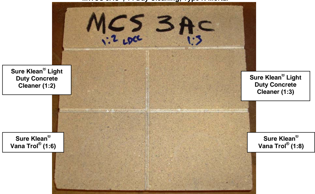
“MWCS 3AC”; 14 Day Cleaning; Type N Mortar
