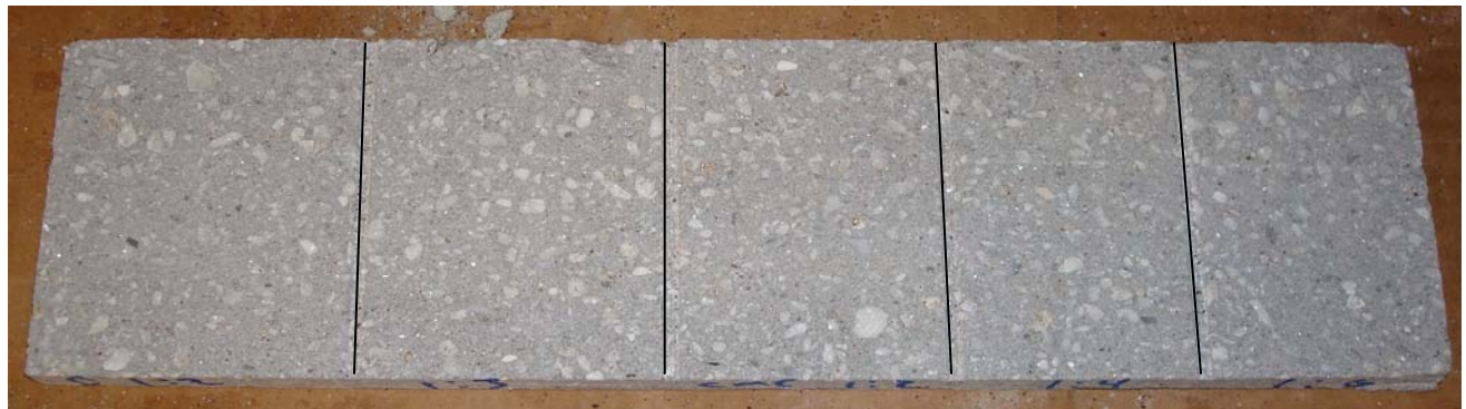
“401” Smooth Finish; 3 Day Cleaning; Type S Mortar
