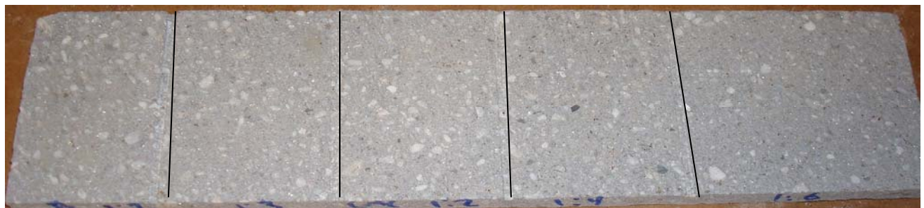
“401” Smooth Finish; 7 Day Cleaning; Type S Mortar
