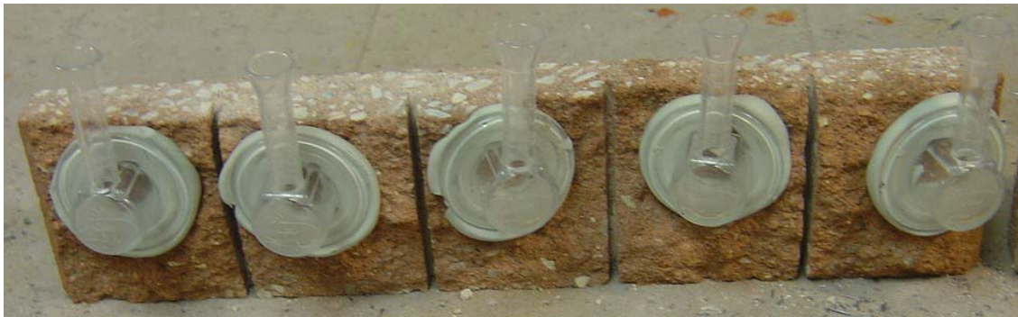
“Deerfield” Split Face CMU; RILEM II.4, 60 mph, 20 Minutes
