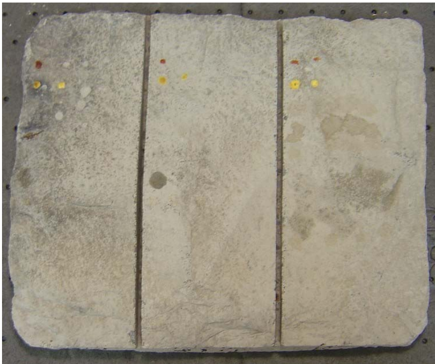
“Chipped Slate”; Stains Removed
