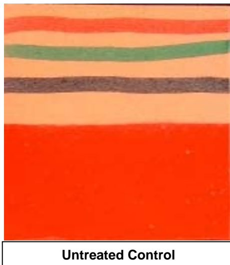
“Sedona Clay – Astra-Glaze-SW+®” Glazed CMU; Before Graffiti Removal
