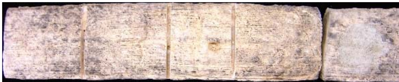
Sure Klean ® Manufactured Stone Cleaner (1:2) Sure Klean ® Manufactured Stone Cleaner (1:3) Enviro Klean ® Safety Klean (1:2) Enviro Klean ® Safety Klean (1:3) Untreated Control
