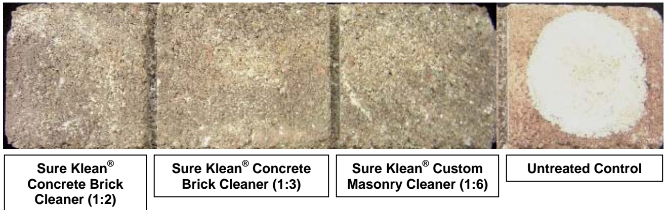
“Niota” Concrete Brick; 21 Day Cleaning
