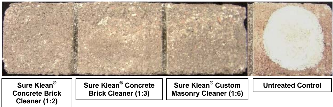
“Niota” Concrete Brick; 14 Day Cleaning
