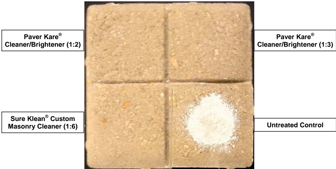
“Warioto Blend” Concrete Paver; 3 Day Cleaning
