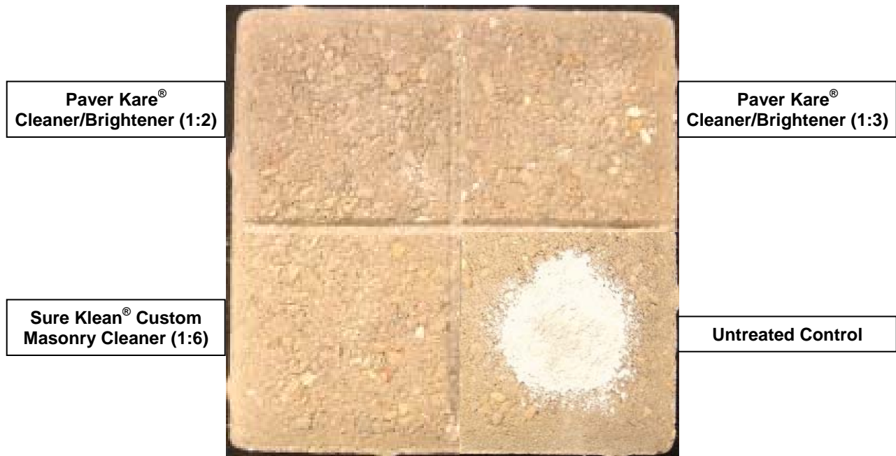
“Warioto Blend” Concrete Paver; 14 Day Cleaning
