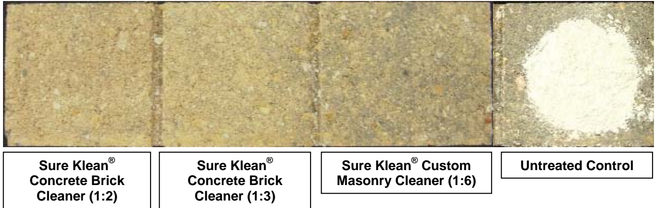
“Smoke” Concrete Brick; 7 Day Cleaning
