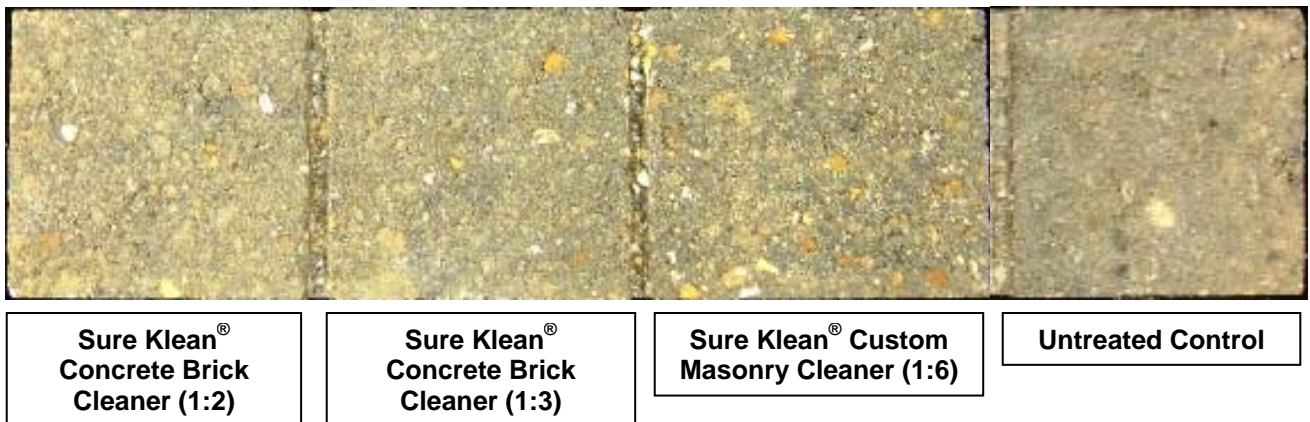
“Smoke” Concrete Brick; Color Uniformity
