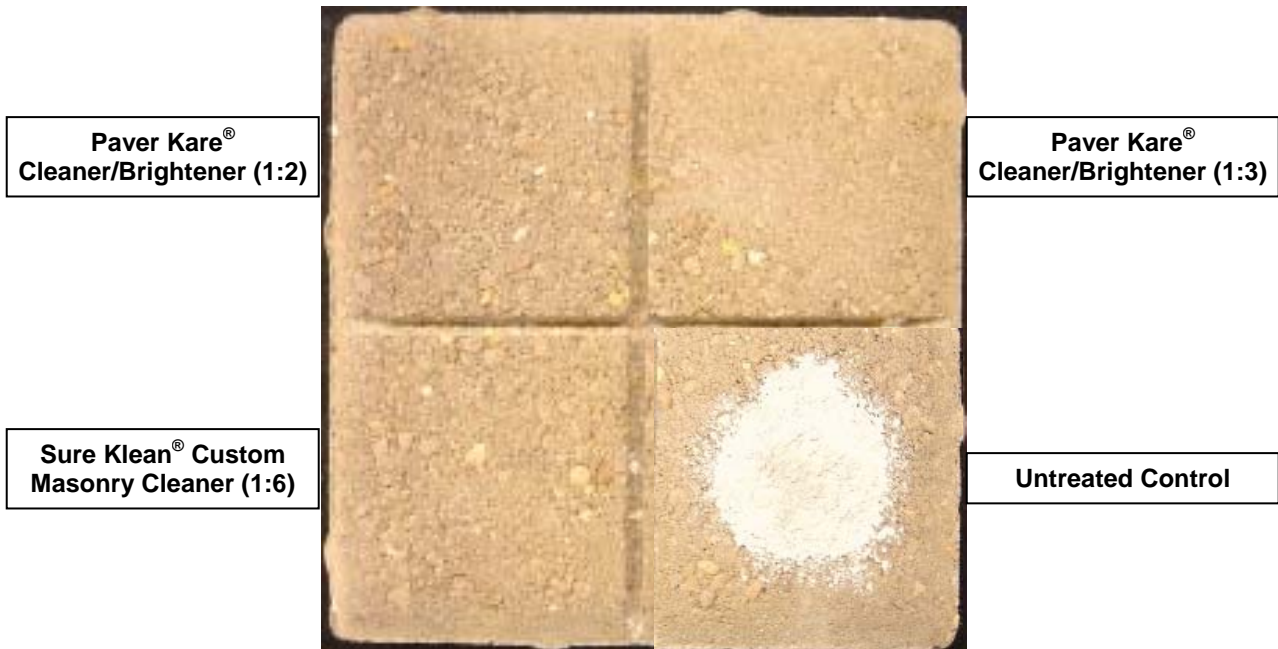
“Warioto Blend” Concrete Paver; 7 Day Cleaning
