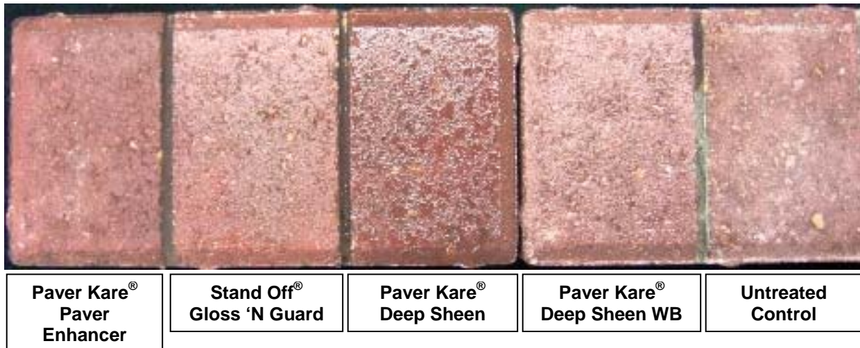
"Red" Concrete Paver; Treatment Applied
