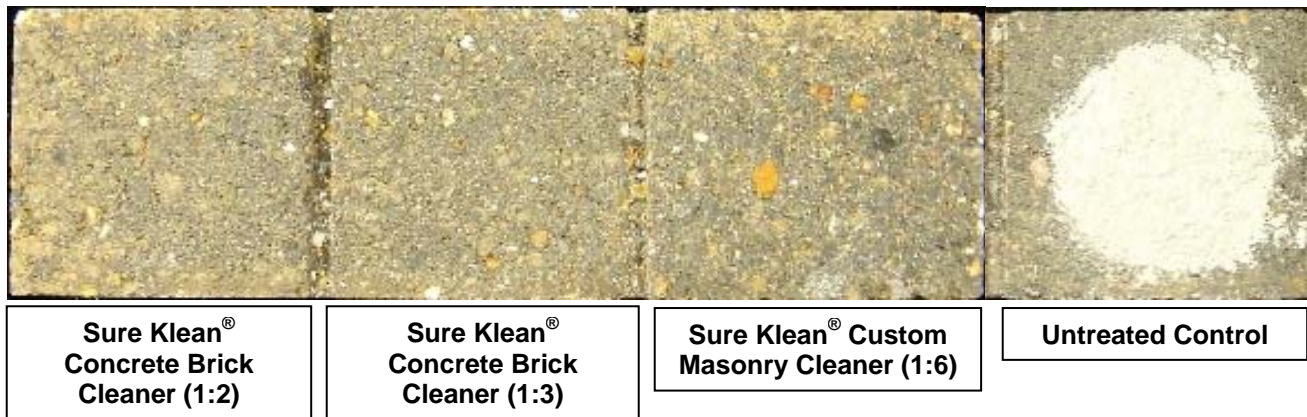
“Smoke” Concrete Brick; 3 Day Cleaning
