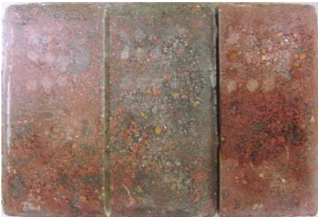
Stand Off ® SLX100 Water & Oil Repellent Stand Off ® Stone, Tile & Masonry Protector (STMP) Untreated Control
