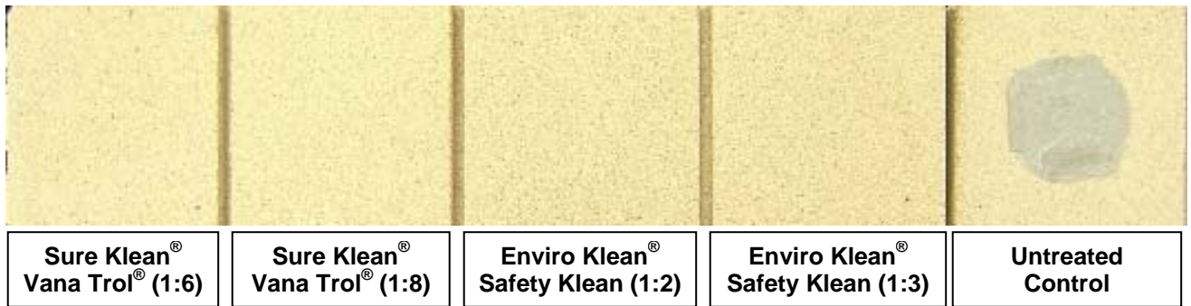
“Limestone”; Type S Mortar; 14 Day Cleaning
