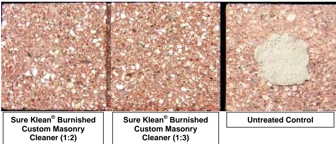
“Old Red” Ground-face CMU; 7 Day Cleaning
