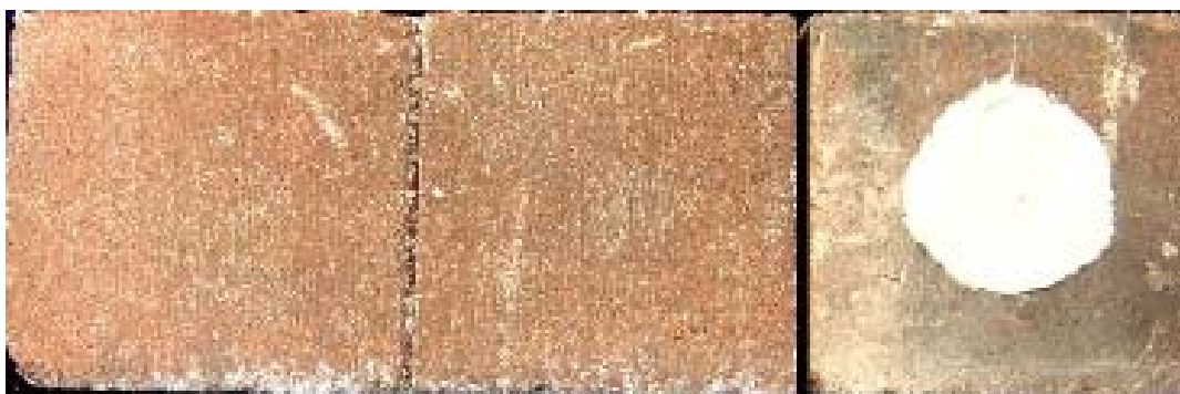
Sure Klean® Concrete Brick Cleaner (1:2) Sure Klean® Concrete Brick Cleaner (1:3) Untreated Control
