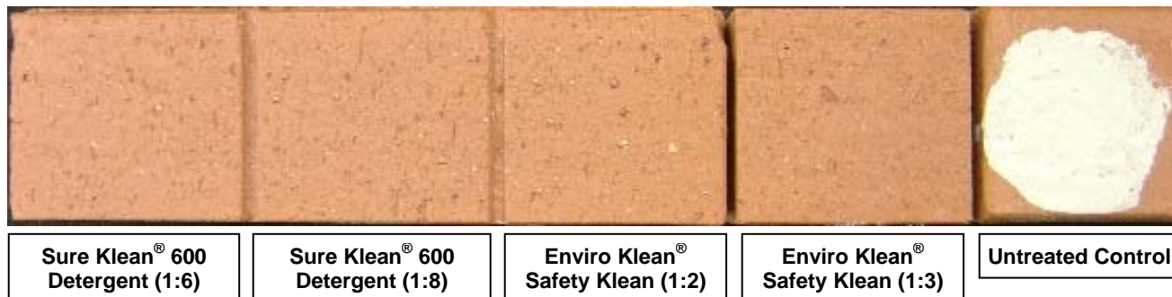
“Dark Red Wire-cut” Clay Brick; 7 Day Cleaning
