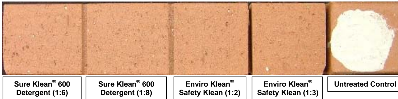
“Dark Red Wire-cut” Clay Brick; 3 Day Cleaning
