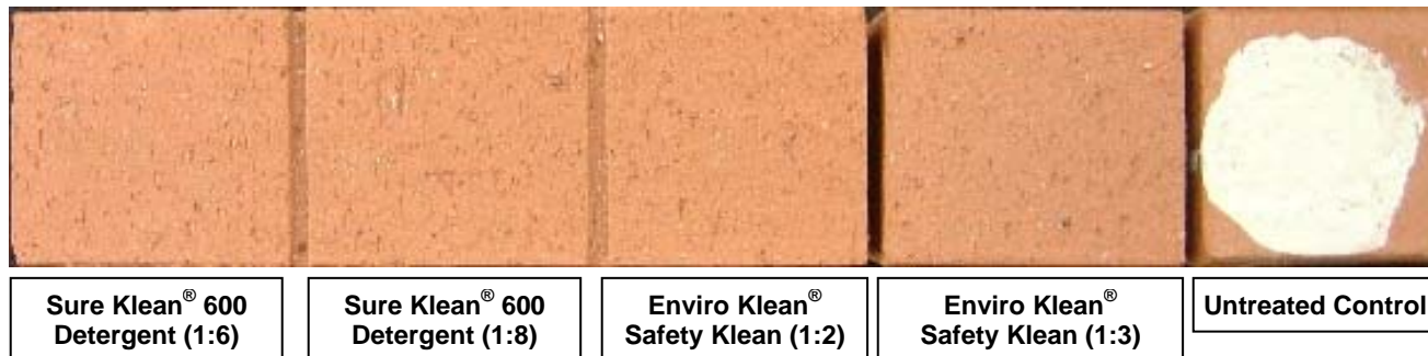
“Dark Red Wire-cut” Clay Brick; 14 Day Cleaning
