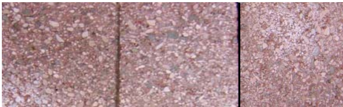
Sure Klean® Burnished Custom Masonry Cleaner (1:2) Sure Klean® Burnished Custom Masonry Cleaner (1:3) Un-cleaned
