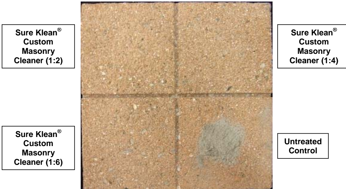
“70D” “Steel Shot Blasted” CMU; 14 Day Cleaning
