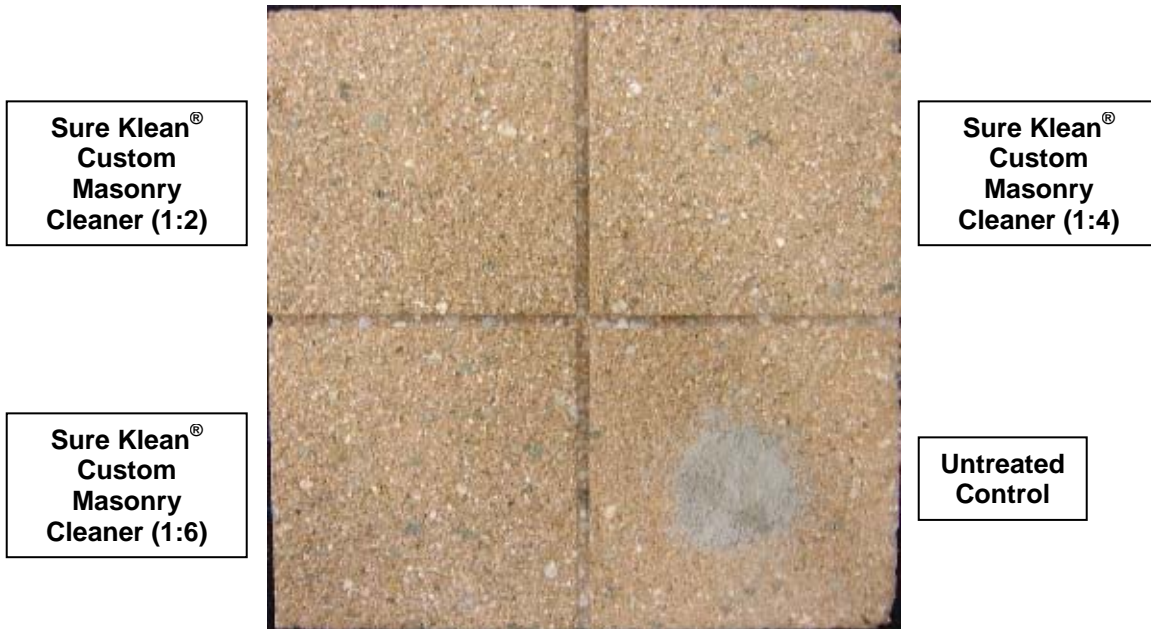
“70D” “Steel Shot Blasted” CMU; 3 Day Cleaning
