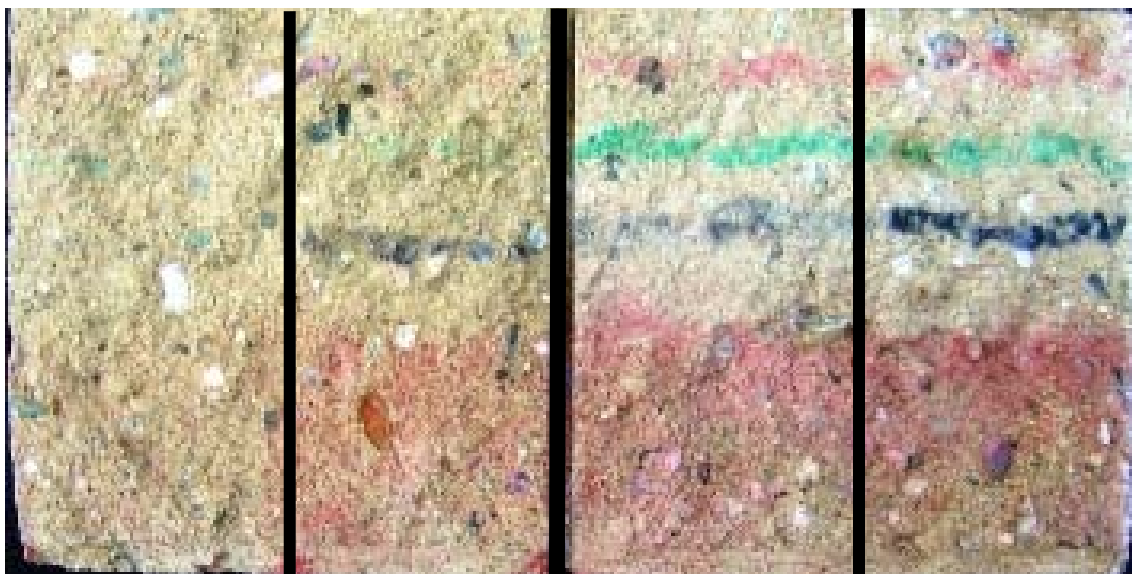
“87” Split-face CMU; After Graffiti Removal
