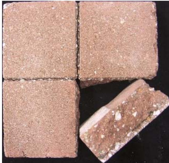
“70D” “Steel Shot Blasted” CMU; Through-body
