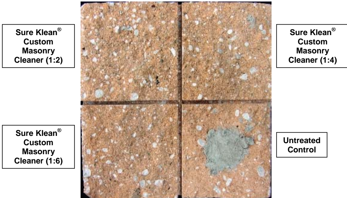
“29” Split-face CMU; 3 Day Cleaning
