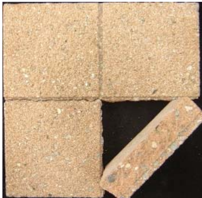
“70D” “Steel Shot Blasted” CMU; Through-body
