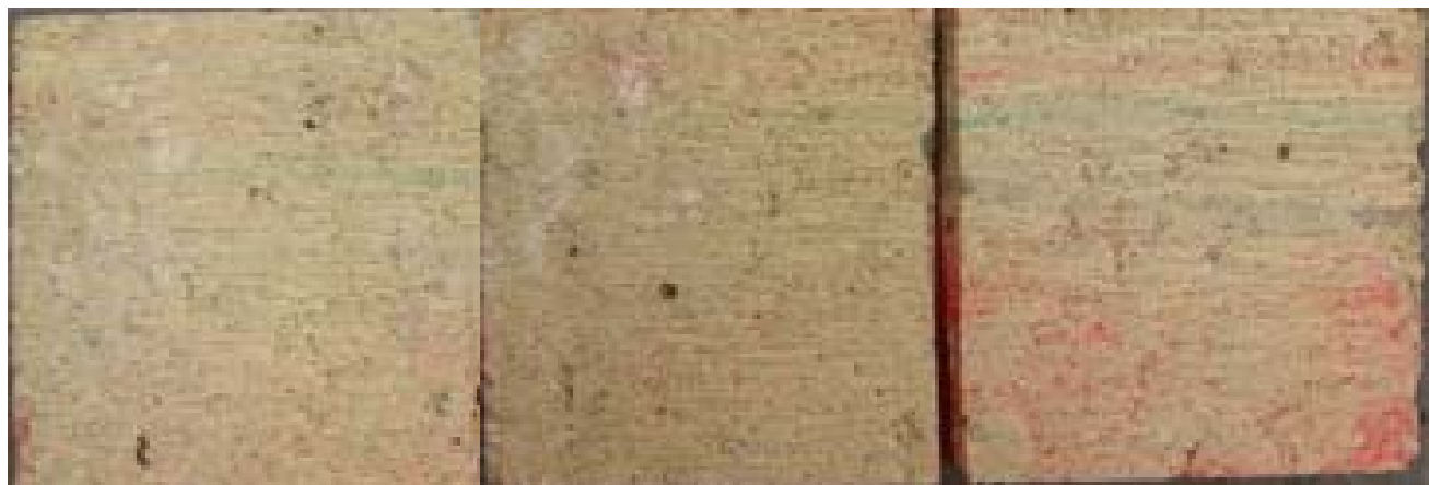
Sure Klean ® Fast Acting Stripper Defacer Eraser ® Graffiti Wipe Sure Klean ® Fast Acting Stripper Defacer Eraser ® Graffiti Wipe Sure Klean ® Fast Acting Stripper Defacer Eraser ® Graffiti Wipe Sure Klean ® Weather Seal Blok-Guard ® & Graffiti Control II Sure Klean ® Weather Seal Blok-Guard ® & Graffiti Control Untreated Control
