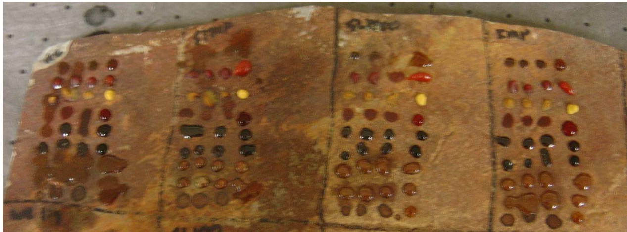
“Wolfcreek Flagstone”; Stains Applied
