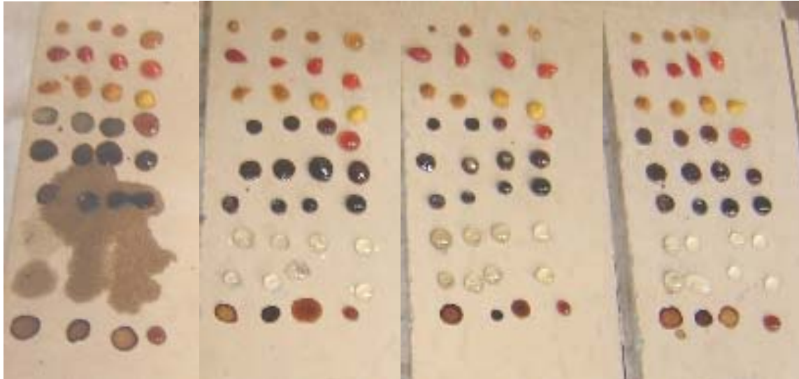
“Granada White” Wall Cap; Stains Applied
