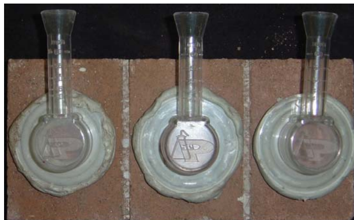
“Red Quick-Brick” CMU - RILEM Testing
