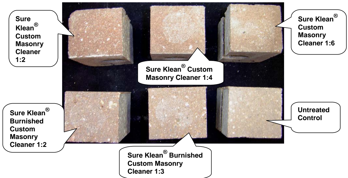
"3" Concrete Brick; 14 Day Cleaning
