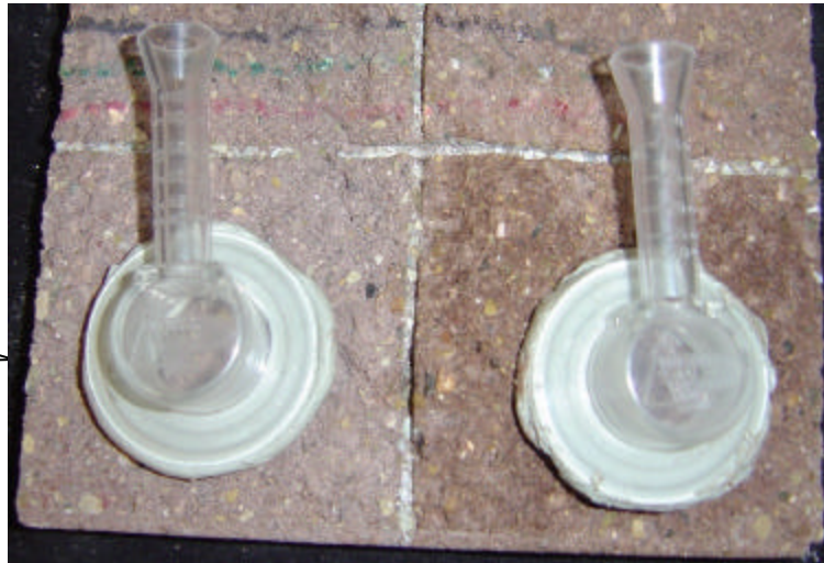
“Canyon Blend” split-face: RILEM testing
