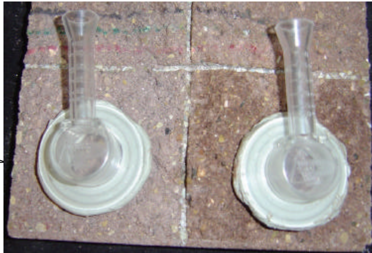
“Canyon Blend” split-face: RILEM testing
