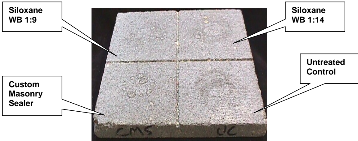
“Granite # 529” Smooth-face block after water repellency treatment
