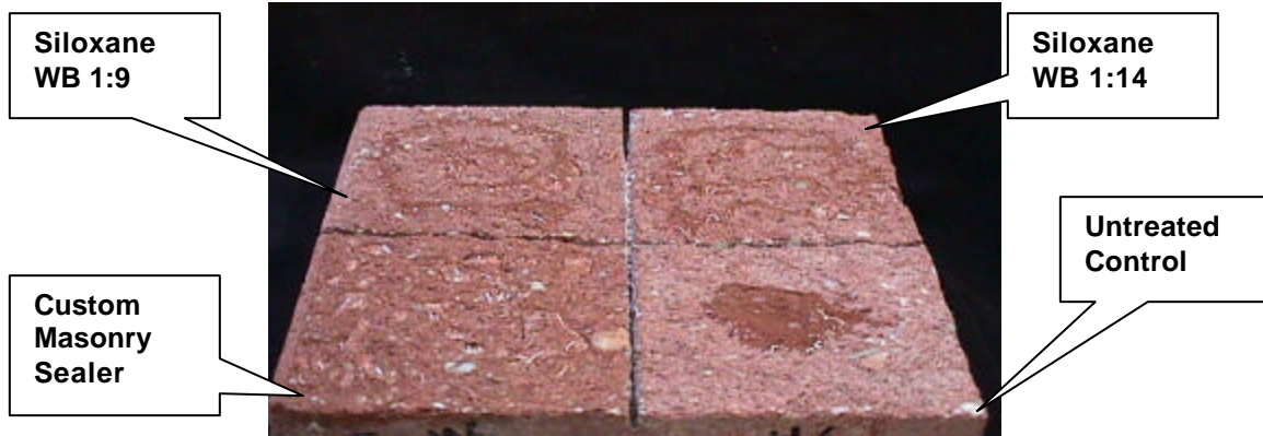
“8SFR” Split-face CMU after water repellency treatment
