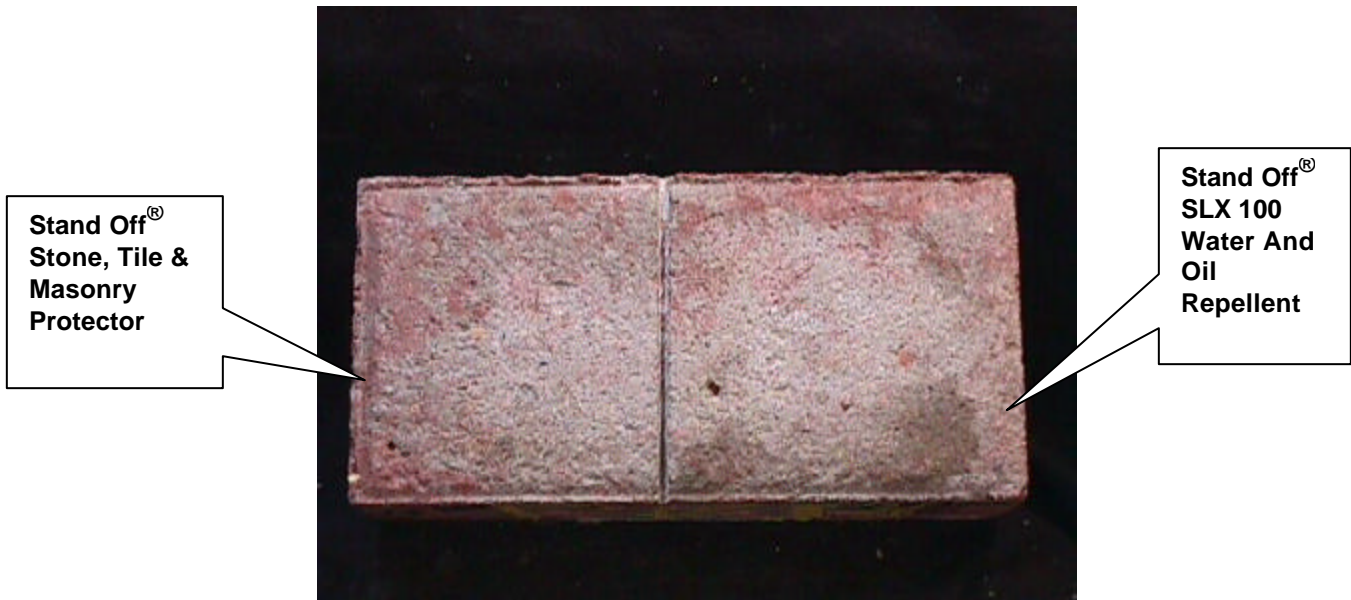
“PBB” Concrete Paver after Cleaning
