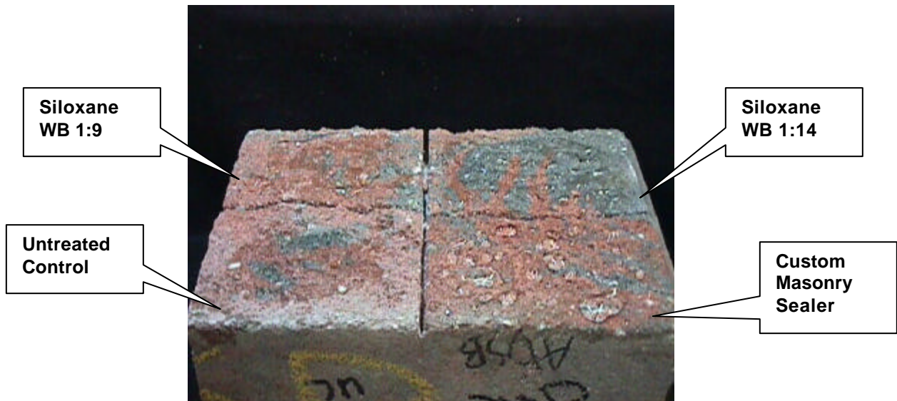
“ADSB” Retaining wall CMU after water repellency treatment
