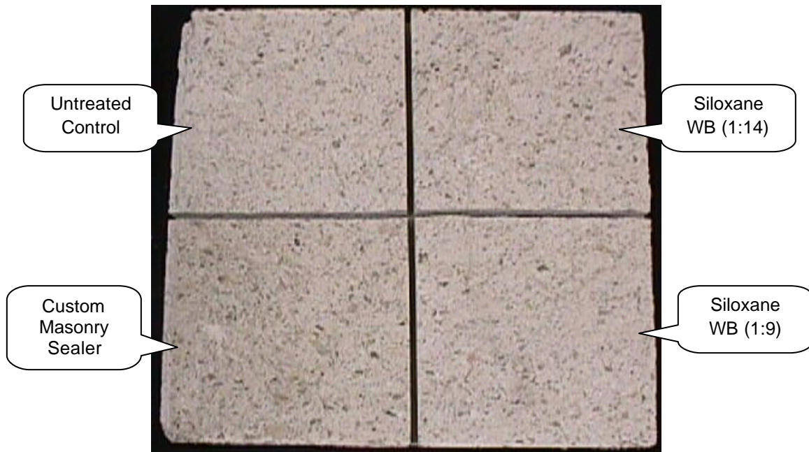
“Arctic White” split-face CMU after water repellency treatment
