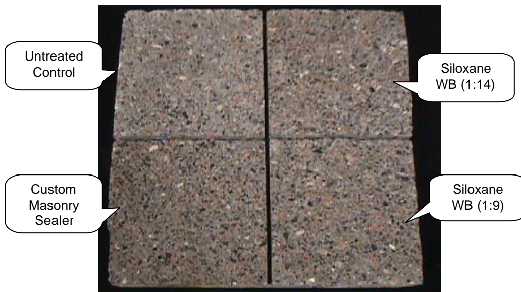
“Lite Weight” split-face CMU after water repellency treatment
