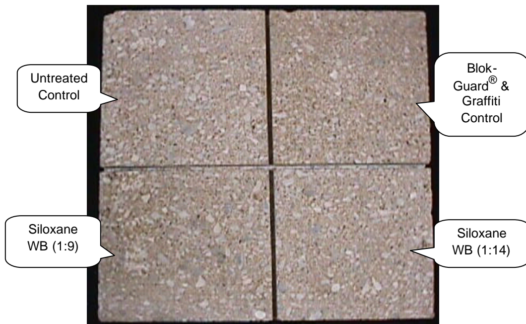
“Old Gold” burnished CMU after water repellency treatment
