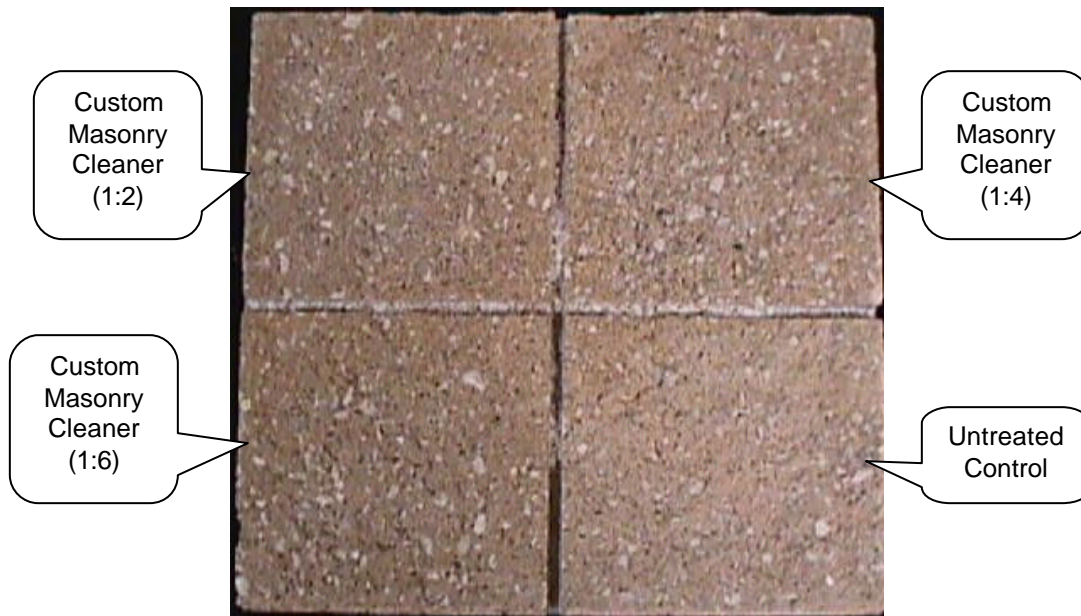
“Buff” Split-face CMU after 14 day cleaning
