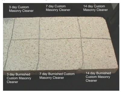
Type "S" Mortar cleaning on Sure Klean® Custom Masonry Sealer
