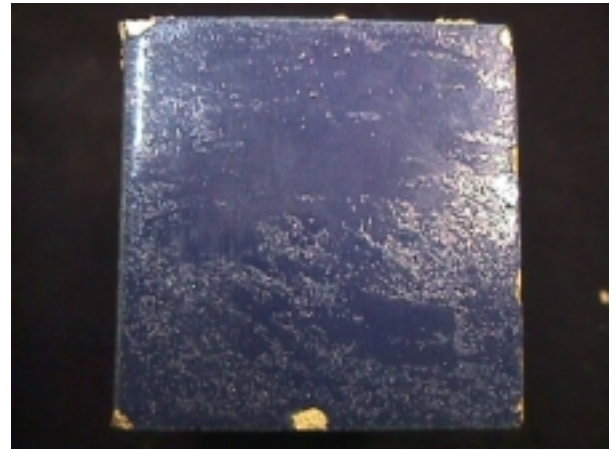
Picture 3.6 – This shows the remaining residual epoxy on the surface of the brick even after 4 – 30 minute dwellings of Fast Acting Stripper on the 14-day cure of 2200A.
