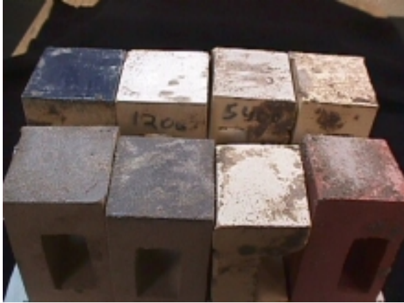
Picture 3.1 - Epoxy grout soiling on all bricks.
