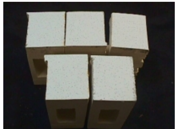
Picture 1.6 – 5400's results of cleaning mortar soiling after a 14-day cure.
