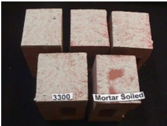
Picture 1.3 – 3300's (Enhanced Engobe) with mortar soiling
