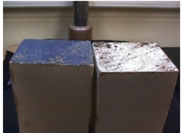
Picture 3.4 - Close-up of epoxy grout soiling of 2200A and 5400.
