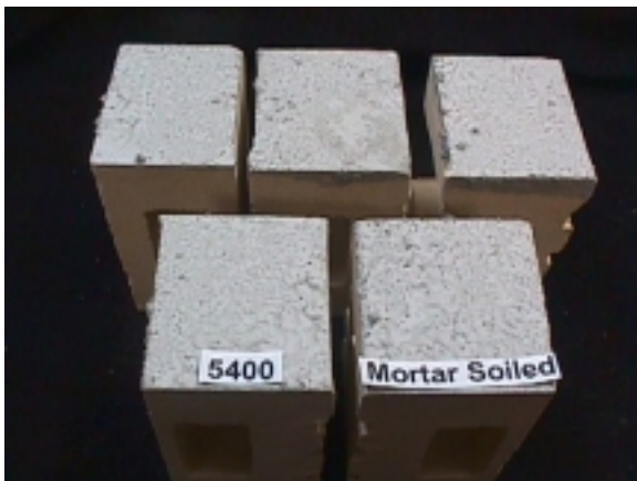
Picture 1.5 – 5400's (Ultra Matte Glaze) with mortar soiling
