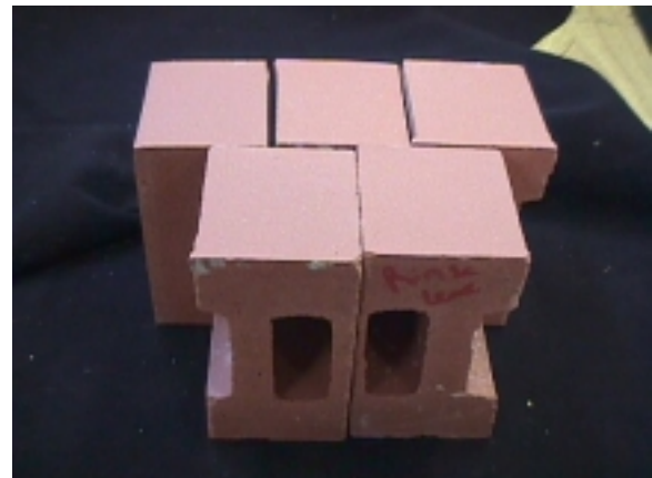
Picture 1.4 – 3300's results of cleaning mortar soiling after a 14-day cure.
