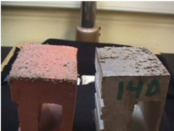
Picture 3.3 – Close-up of epoxy grout soiling on 3300 and 4435.
