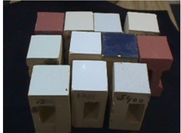
Picture 3.2 - Epoxy grout successfully removed from bricks.
