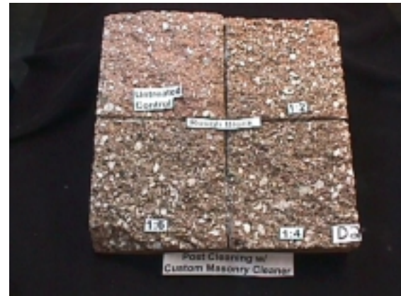
Cocoa rough block post cleaning with CMC
