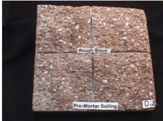
Cocoa rough block prior to mortar soiling
