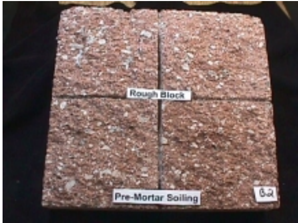
Burnt Orange rough block prior to mortar soiling
