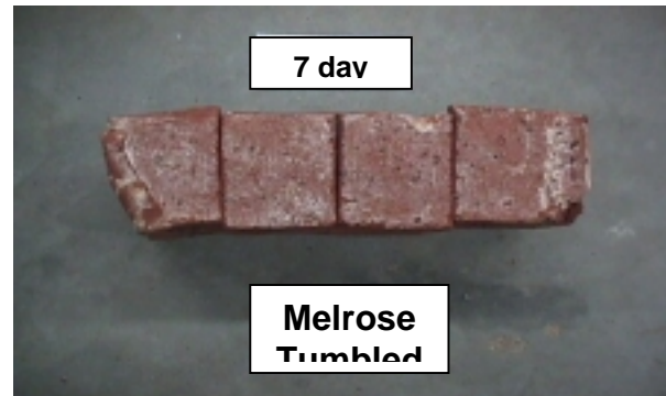
AFTER 7 day MORTAR CLEANING
