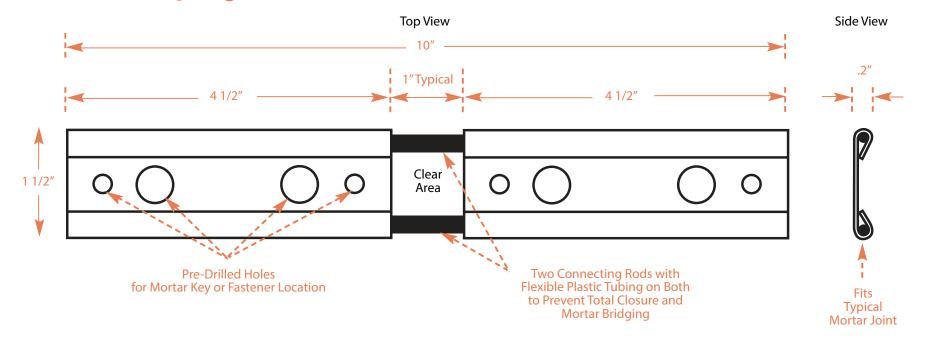
Expansion Joint Stabilizer \_\_\_\_\_ Stainless Steel Sheet per ASTM A-167, Type 304 or
