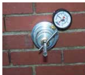
Pull-Out Capacity Brick
