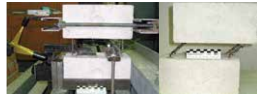
CTP Stitch-Tie testing for shelf angle support
