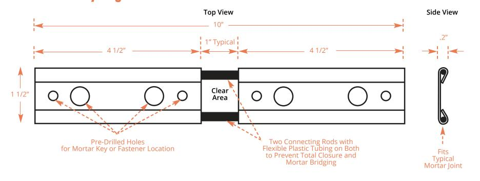
CTP MAD-2000 \_\_\_\_\_ Stainless Steel Sheet per ASTM A-167, Type 304 or
