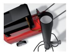
6. Pour the mix into a pneumatic grout gun, connected to a compressor - set to a maximum of 3 bar (44psi) pressure.
