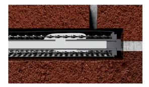
8. The HDS Sock Anchor system is back-filled, expanding the reinforced mesh sock to completely fill any voids, providing a permanent cementitious fixing to the surrounding masonry.
