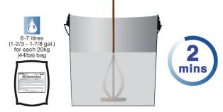
5. To mix the grout, add the appropriate amount of water first, then the powder and mix well using a paddle, until a very fluid but creamy uniform consistency is created. Always maintain the correct working ratio, as per the manufacturer's instructions.
