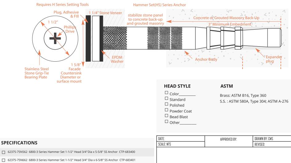
C 62375-75N572 6800-3 Series Hammer Set 1-1/2" Head 3/4" Dia x 7-5/8" SS Anchor CTP-683402
