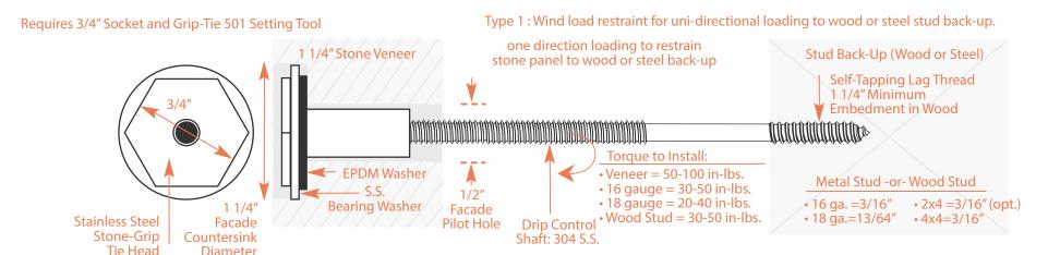
• S.S : ASTM 580A, Type 304; ASTM A-276
