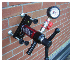
Mortar Joint Performance Test
