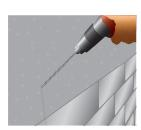
Step 1: Drill a 3/16" pilot hole using a percussion hammer drill (3-jaw-chuck type) through the stucco.
